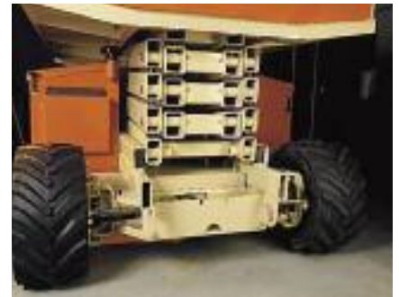
Strengthened Arm Stack for Improved Stack Rigidity
