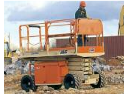
Standard Cross Corner Four-Wheel Drive for Terrainability
