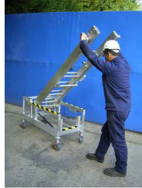
3. Raise mast to 45° position & engage bolts
