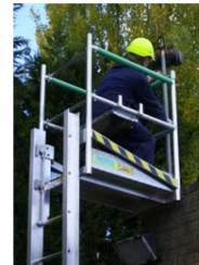
17. Always keep your body within the guardrailed platform area. Reach out with arms and hands only. Do not stretch. Do not overload the DESKSURFER. The Maximum Safe Working Load is 150kg (23.5 stone).
