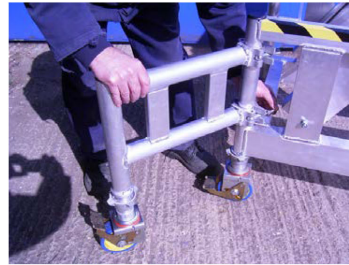
9. Couple on 4no. outriggers 2no. Front & 2no. Rear outriggers @ 45° position and tighten wing nuts (also see instruction no.12)
