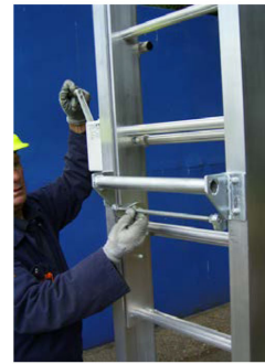
14. To raise mast insert handle (stored in base frame) into the winch box.
